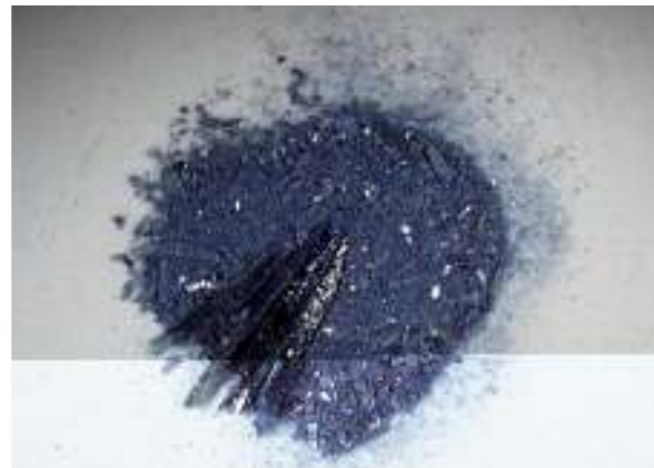
Fig. 4 Vivianite from the Ukraine Pulverised blackish-blue clump of vivianite, which resulted in an intense indigo-like blue pigment
